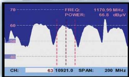
High resolution Spectrum Analyser with direct access keys
