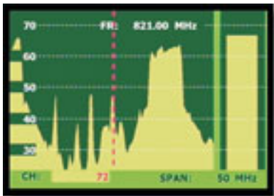
Antenna alignment screen
