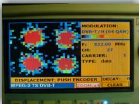
Isti 64 QAM signal pod pove alom, ZOOM x 4
