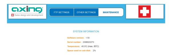
In the system information area, the installed software version, the serial number, the temperature of the device and the percentage of the space used on the connected USB stick are displayed.
