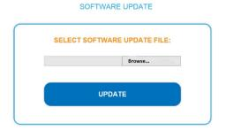
To update the software of the device, select the corresponding file (softa.zip) on a data carrier using the "Browse..." button and then press "Update".
