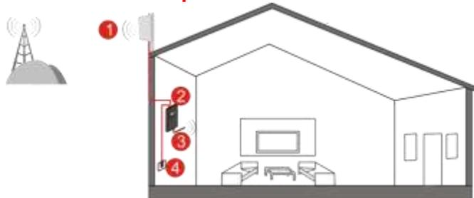
1. Outdoor Antenna    2. Booster    3. Indoor Antenna    4. Power Supply
