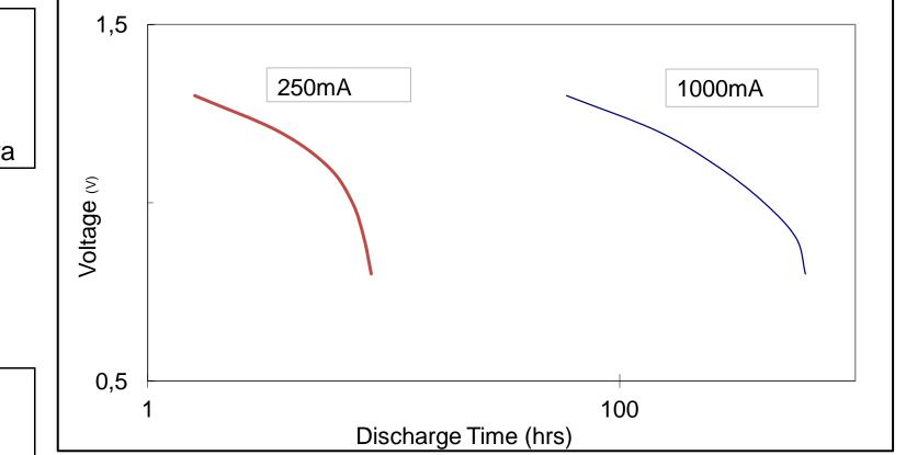
Test environment: 20  $^{\circ}$ C  $\pm$  2,60%  $\pm$  15% R.H, Load resistance: 3.9 ohms, time: 0.3s
